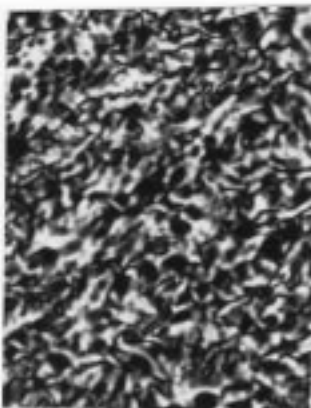
Figure 2. Evolution of mesophase structure at the 20/80 K36/s-SCLCP composition during the course of (a) cooling and (b) heating cycles, showing a reversible phase change from isotropic, isotropic + nematic, and the pure nematic. The ramp rate was 0.5 °C/min.
